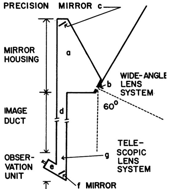
Fig. 1. Diagram of periscopic system for observation of behavior.
